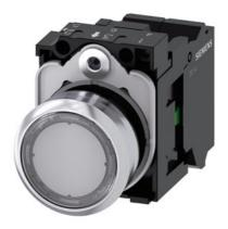
Illuminated pushbutton, 22 mm, round, Metal, shiny, transparent, pushbutton, flat, momentary contact type, with holder, 1NO, LED module with integrated LED 230 V AC, spring-type terminal, with laser labeling, upper case and lower case, always upper case at the beginning of the word
