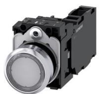
Illuminated pushbutton, 22 mm, round, metal, shiny, clear, pushbutton, flat, momentary contact type, with holder, 1 NO+1 NC, LED module with integrated LED 230 V AC, screw terminal
