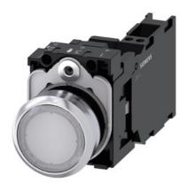
Illuminated pushbutton, 22 mm, round, Metal, shiny, white, pushbutton, flat, momentary contact type, with holder, 1 NO+1 NC, LED module with integrated LED 230 V AC, spring-type terminal, with laser labeling, upper case
