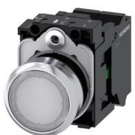
Illuminated pushbutton, 22 mm, round, metal, shiny, white, pushbutton, flat, momentary contact type, with holder, 1 NO, LED module with integrated LED 230 V AC, Spring-type terminal
