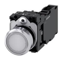
Illuminated pushbutton, 22 mm, round, Metal, shiny, white, pushbutton, flat, momentary contact type, with holder, 1 NO+1 NC, LED module with integrated LED 230 V AC, screw terminal, with laser labeling, lower case
