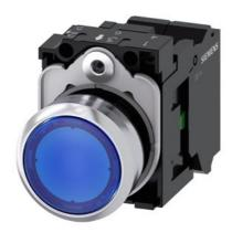
Illuminated pushbutton, 22 mm, round, Metal, shiny, blue, pushbutton, flat, momentary contact type, with holder, 1NO, LED module with integrated LED 230 V AC, spring-type terminal, with laser labeling, upper case and lower case, always upper case at beginning of line
