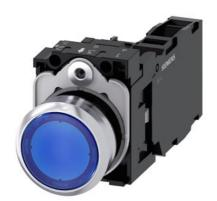
Illuminated pushbutton, 22 mm, round, Metal, shiny, blue, pushbutton, flat, momentary contact type, with holder, 1 NO+1 NC, LED module with integrated LED 230 V AC, screw terminal, with laser labeling, inscription or symbol Customer-specific selection with SIRIUS ACT configurator (CIN)
