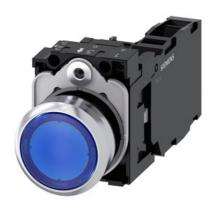
Illuminated pushbutton, 22 mm, round, Metal, shiny, blue, pushbutton, flat, momentary contact type, with holder, 1 NO+1 NC, LED module with integrated LED 230 V AC, screw terminal, with laser labeling, upper case and lower case, always upper case at the beginning of the word
