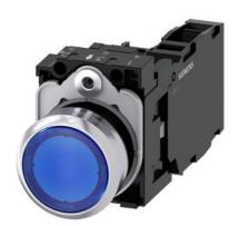
Illuminated pushbutton, 22 mm, round, Metal, shiny, blue, pushbutton, flat, momentary contact type, with holder, 1 NO+1 NC, LED module with integrated LED 230 V AC, screw terminal, with laser labeling, symbol number according to, ISO 7000 or IEC 60417
