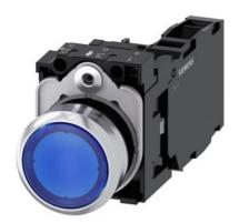
Illuminated pushbutton, 22 mm, round, metal, shiny, blue, pushbutton, flat, momentary contact type, with holder, 1 NO+1 NC, LED module with integrated LED 230 V AC, screw terminal, Z=20-unit packaging
