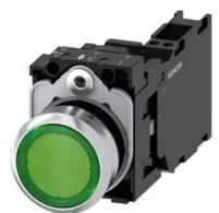
Illuminated pushbutton, 22 mm, round, metal, shiny, green, pushbutton, flat, momentary contact type, with holder, 1 NO+1 NC, LED module with integrated LED 230 V AC, Spring-type terminal
