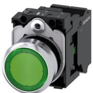
Illuminated pushbutton, 22 mm, round, Metal, shiny, green, pushbutton, flat, momentary contact type, with holder, 1NO, LED module with integrated LED 230 V AC, spring-type terminal, with laser labeling, upper case and lower case, always upper case at beginning of line
