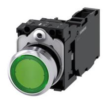
Illuminated pushbutton, 22 mm, round, Metal, shiny, green, pushbutton, flat, momentary contact type, with holder, 1 NO+1 NC, LED module with integrated LED 230 V AC, screw terminal, with laser labeling, upper case
