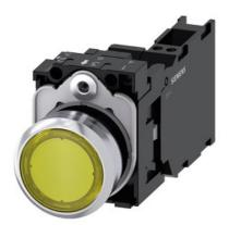
Illuminated pushbutton, 22 mm, round, Metal, shiny, yellow, pushbutton, flat, momentary contact type, with holder, 1 NO+1 NC, LED module with integrated LED 230 V AC, spring-type terminal, with laser labeling, lower case
