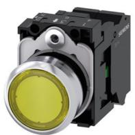
Illuminated pushbutton, 22 mm, round, Metal, shiny, yellow, pushbutton, flat, momentary contact type, with holder, 1NO, LED module with integrated LED 230 V AC, spring-type terminal, with laser labeling, inscription or symbol Customer-specific selection with SIRIUS ACT configurator (CIN)
