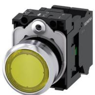
Illuminated pushbutton, 22 mm, round, metal, shiny, yellow, pushbutton, flat, momentary contact type, with holder, 1NO, LED module with integrated LED 230 V AC, spring-type terminal, Z=20-unit packaging
