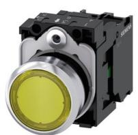
Illuminated pushbutton, 22 mm, round, metal, shiny, yellow, pushbutton, flat, momentary contact type, with holder, 1 NO, LED module with integrated LED 230 V AC, screw terminal
