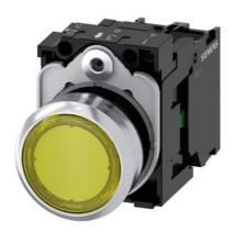
Illuminated pushbutton, 22 mm, round, Metal, shiny, yellow, pushbutton, flat, momentary contact type, with holder, 1NO, LED module with integrated LED 230 V AC, screw terminal, with laser labeling, symbol number according to, ISO 7000 or IFC 60417
