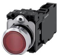
Illuminated pushbutton, 22 mm, round, metal, shiny, red, pushbutton, flat, momentary contact type, with holder, 1 NO+1 NC, LED module with integrated LED 230 V AC, screw terminal
