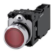
Illuminated pushbutton, 22 mm, round, Metal, shiny, red, pushbutton, flat, momentary contact type, with holder, 1 NO+1 NC, LED module with integrated LED 230 V AC, screw terminal, with laser labeling, symbol number according to, ISO 7000 or IEC 60417
