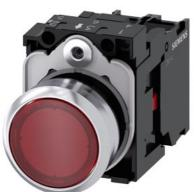
Illuminated pushbutton, 22 mm, round, metal, shiny, red, pushbutton, flat, momentary contact type, with holder, 1 NC, LED module with integrated LED 230 V AC, screw terminal
