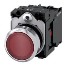
Illuminated pushbutton, 22 mm, round, metal, shiny, red, pushbutton, flat, momentary contact type, with holder, 1NC, LED module with integrated LED 230 V AC, screw terminal, with laser labeling, upper case and lower case, always upper case at beginning of line
