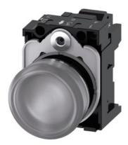
Indicator lights, 22 mm, round, metal, shiny, clear, lens, smooth, with holder, LED module with integrated LED 110 V AC, spring-type terminal, with laser labeling, upper case and lower case, always upper case at the beginning of the word
