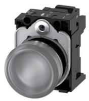
Indicator light, 22 mm, round, metal, shiny, clear, lens, smooth, with holder, LED module with integrated LED 110 V AC, spring-type terminal, with laser labeling, upper case and lower case, always upper case at beginning of line
