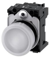
Indicator lights, 22 mm, round, metal, shiny, white, lens, smooth, with holder, LED module with integrated LED 110 V AC, screw terminal, with laser labeling, inscription or symbol Customer-specific selection with SIRIUS ACT configurator (CIN)
