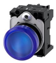
Indicator light, 22 mm, round, metal, shiny, blue, lens, smooth, with holder, LED module with integrated LED 110 V AC, screw terminal, with laser labeling, upper case and lower case, always upper case at beginning of line
