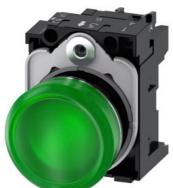
Indicator lights, 22 mm, round, metal, shiny, green, lens, smooth, with holder, LED module with integrated LED 110 V AC, screw terminal, with laser labeling, upper case
