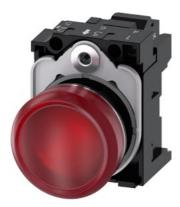
Indicator lights, 22 mm, round, metal, shiny, red, lens, smooth, with holder, LED module with integrated LED 110 V AC, spring-type terminal, with laser labeling, inscription or symbol Customer-specific selection with SIRIUS ACT configurator (CIN)
