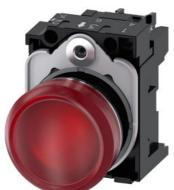
Indicator lights, 22 mm, round, metal, shiny, red, lens, smooth, with holder, LED module with integrated LED 110 V AC, screw terminal, with laser labeling, lower case
