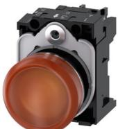
Indicator lights, 22 mm, round, metal, shiny, amber, lens, smooth, with holder, LED module with integrated LED 110 V AC, screw terminal, with laser labeling, lower case
