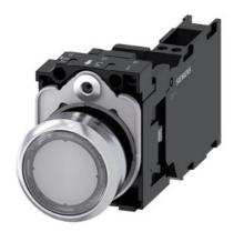
Illuminated pushbutton, 22 mm, round, metal, shiny, clear, pushbutton, flat, momentary contact type, with holder, 1 NO+1 NC, LED module with integrated LED 110 V AC, Spring-type terminal
