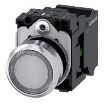
Illuminated pushbutton, 22 mm, round, metal, shiny, clear, pushbutton, flat, momentary contact type, with holder, 1 NO, LED module with integrated LED 110 V AC, Spring-type terminal
