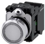
Illuminated pushbutton, 22 mm, round, metal, shiny, clear, pushbutton, flat, momentary contact type, with holder, 1NO, LED module with integrated LED 110 V AC, spring-type terminal, with laser labeling, upper case and lower case, always upper case at beginning of line
