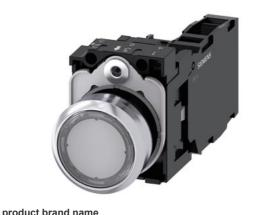
Illuminated pushbutton, 22 mm, round, metal, shiny, clear, pushbutton, flat, momentary contact type, with holder, 1 NO+1 NC, LED module with integrated LED 110 V AC, screw terminal
