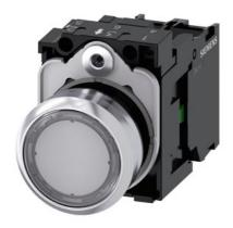
Illuminated pushbutton, 22 mm, round, metal, shiny, clear, pushbutton, flat, momentary contact type, with holder, 1 NO, LED module with integrated LED 110 V AC. screw terminal
