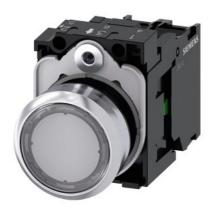
Illuminated pushbutton, 22 mm, round, metal, shiny, clear, pushbutton, flat, momentary contact type, with holder, 1NO, LED module with integrated LED 110 V AC, screw terminal, with laser labeling, lower case
