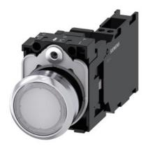
Illuminated pushbutton, 22 mm, round, metal, shiny, white, pushbutton, flat, momentary contact type, with holder, 1 NO+1 NC, LED module with integrated LED 110 V AC, Spring-type terminal
