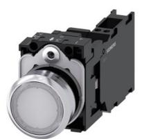
Illuminated pushbutton, 22 mm, round, metal, shiny, white, pushbutton, flat, momentary contact type, with holder, 1 NO+1 NC, LED module with integrated LED 110 V AC, spring-type terminal, with laser labeling, inscription or symbol Customer-specific selection with SIRIUS ACT configurator (CIN)
