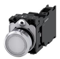
Illuminated pushbutton, 22 mm, round, metal, shiny, white, pushbutton, flat, momentary contact type, with holder, 1 NO+1 NC, LED module with integrated LED 110 V AC, spring-type terminal, with laser labeling, symbol number according to, ISO 7000 or IEC 60417
