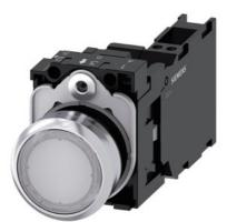
Illuminated pushbutton, 22 mm, round, metal, shiny, white, pushbutton, flat, momentary contact type, with holder, 1 NO+1 NC, LED module with integrated LED 110 V AC, spring-type terminal, Z=20-unit packaging
