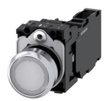
Illuminated pushbutton, 22 mm, round, metal, shiny, white, pushbutton, flat, momentary contact type, with holder, 1 NO+1 NC, LED module with integrated LED 110 V AC, screw terminal, with laser labeling, inscription or symbol Customer-specific selection with SIRIUS ACT configurator (CIN)
