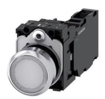
Illuminated pushbutton, 22 mm, round, metal, shiny, white, pushbutton, flat, momentary contact type, with holder, 1 NO+1 NC, LED module with integrated LED 110 V AC, screw terminal, with laser labeling, upper case and lower case, always upper case at beginning of line
