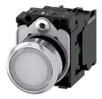
Illuminated pushbutton, 22 mm, round, metal, shiny, white, pushbutton, flat, momentary contact type, with holder, 1 NO, LED module with integrated LED 110 V AC. screw terminal
