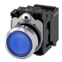
Illuminated pushbutton, 22 mm, round, metal, shiny, blue, pushbutton, flat, momentary contact type, with holder, 1NO, LED module with integrated LED 110 V AC, spring-type terminal, with laser labeling, upper case
