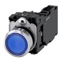
Illuminated pushbutton, 22 mm, round, metal, shiny, blue, pushbutton, flat, momentary contact type, with holder, 1 NO+1 NC, LED module with integrated LED 110 V AC, screw terminal, with laser labeling, upper case and lower case, always upper case at beginning of line
