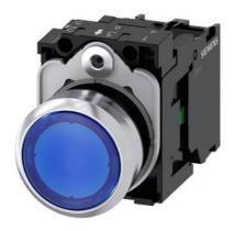
Illuminated pushbutton, 22 mm, round, metal, shiny, blue, pushbutton, flat, momentary contact type, with holder, 1 NO, LED module with integrated LED 110 V AC. screw terminal
