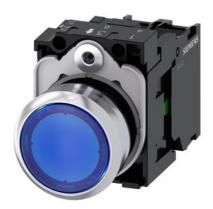
Illuminated pushbutton, 22 mm, round, metal, shiny, blue, pushbutton, flat, momentary contact type, with holder, 1NO, LED module with integrated LED 110 V AC, screw terminal, Z=20-unit packaging
