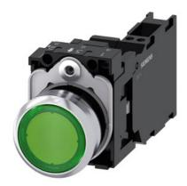
Illuminated pushbutton, 22 mm, round, metal, shiny, green, pushbutton, flat, momentary contact type, with holder, 1 NO+1 NC, LED module with integrated LED 110 V AC, Spring-type terminal
