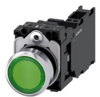
Illuminated pushbutton, 22 mm, round, metal, shiny, green, pushbutton, flat, momentary contact type, with holder, 1 NO+1 NC, LED module with integrated LED 110 V AC, spring-type terminal, with laser labeling, symbol number according to, ISO 7000 or IEC 60417
