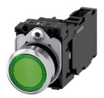
Illuminated pushbutton, 22 mm, round, metal, shiny, green, pushbutton, flat, momentary contact type, with holder, 1 NO+1 NC, LED module with integrated LED 110 V AC, screw terminal, with laser labeling, upper case and lower case, Always upper case at the beginning of the word
